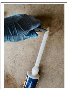
**Step 4**. Squeeze 2 inches out before using the product. You do not want to apply epoxy that hasn't mixed. It will not set up. The nozzle is designed to mix the epoxy by the time it is out but this assures that it is mixed for use. The tube is designed with 2 compartments and the product is pushed out evenly from both compartments.
